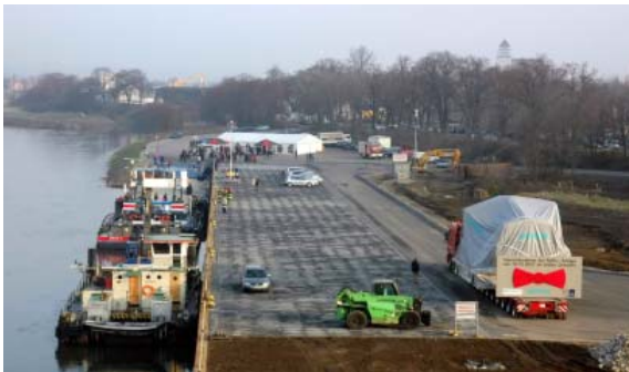
A turbine from the Siemens turbine works in Görlitz was the first item of heavy freight to be loaded using the ro-ro facility
